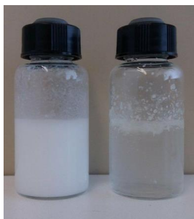
Figure 15: Photograph showing the visual aspect of vials containing empty nanoparticles (left) or loaded nanoparticles with tobramycin after 1 month (right).
